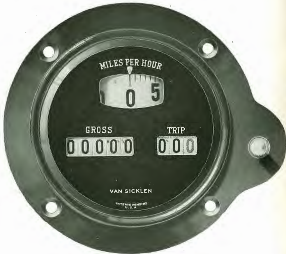
FLUSH TYPE, KNURLED RESET, BLACK FACE, NICKLE OR BLACK BEZEL
