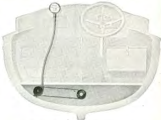
This illustration shows Revolution Indicator mounted on dash and connected to propeller shaft
